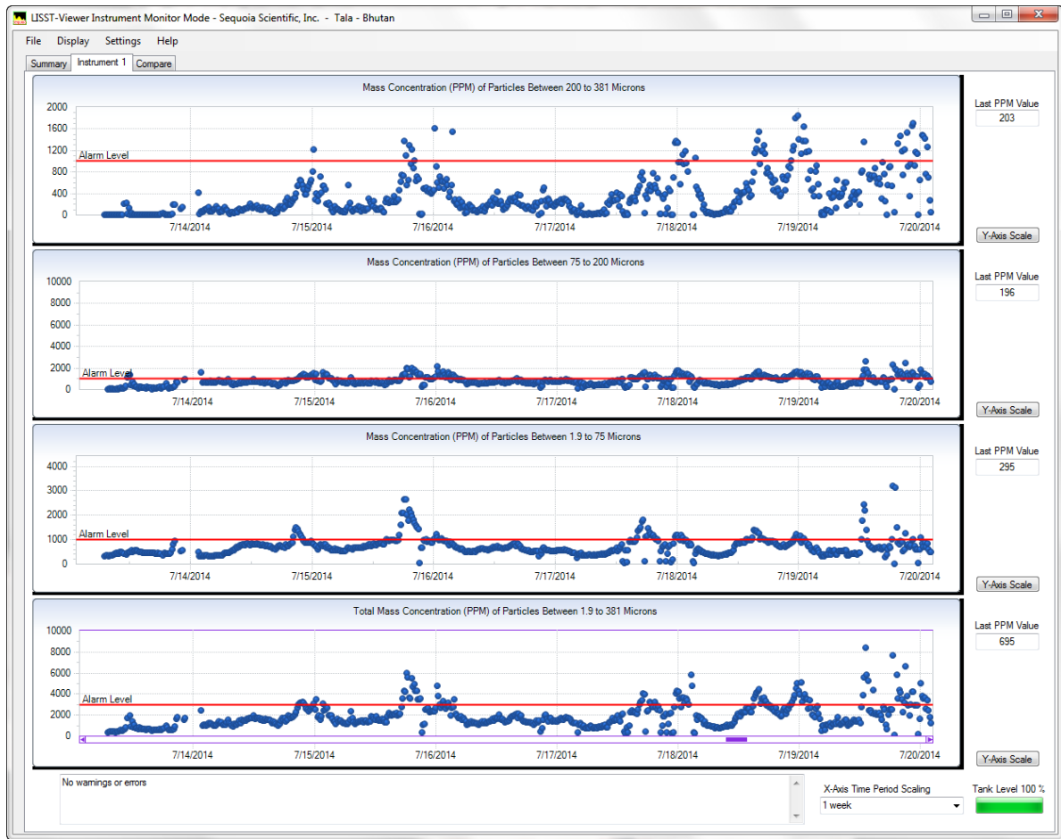
Figure 5: Strip chart display of history of concentrations for a single instrument. The charts show concentrations in, from bottom to top, all, fine (<75), medium (75 to 200) and coarse (>200 \mu\text{m} ) fractions. [note: the alarm levels are set extremely low here; the operator was playing.]
